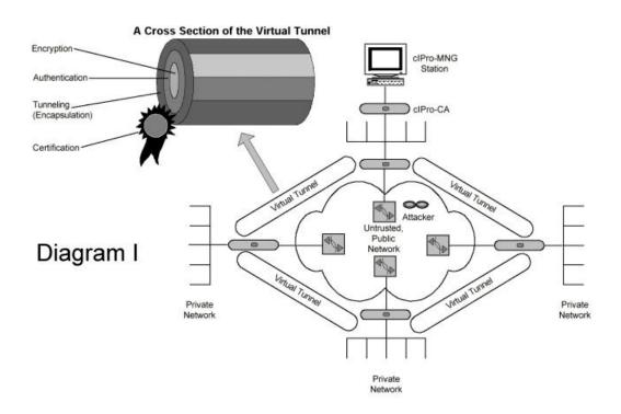
Within this secure VPN, data passed from one device to another flows through the public network through a multi-layer "virtual tunnel" of security algorithms (in the diagram the virtual tunnels are separated from the public network to demonstrate their isolation from the
